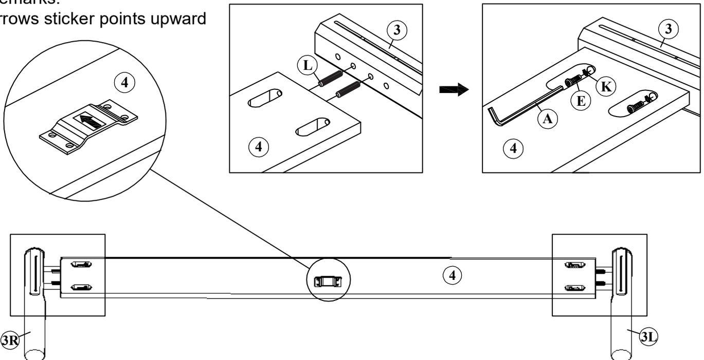
STEP 3 : Attach (5) to Assembled Headboard and Footboard as shown.
